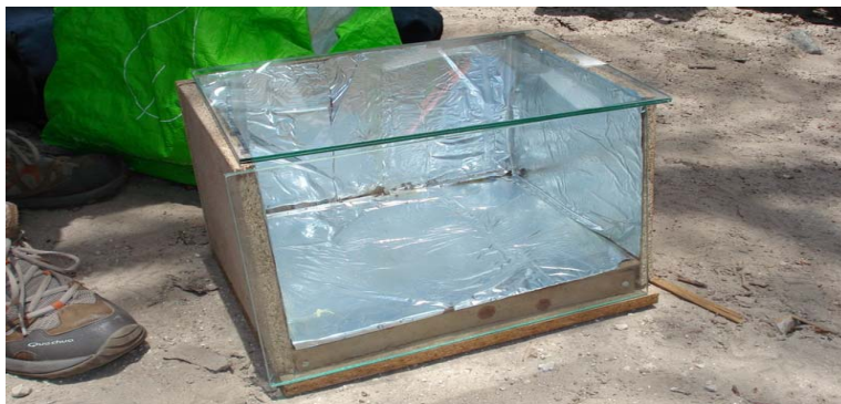
solar oven capable of reaching 70°C
