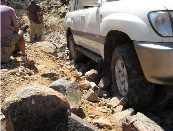
We managed to get the other trucks up after much careful line picking and rock climbing but the cruiser double cab with the defective diff lock and bike trailer was not coming up. After unhitching the trailer and lowering tire pressures to 1.2 bar the double cab crawled out. We then had to man handle the trailer up that rocky slope. Not an exercise we want to repeat again especially as it was 40+.
